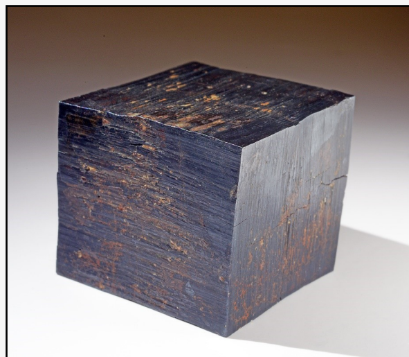
FIGURE N PSEUDOMORPH This is a pyrite cube that has been replaced by limonite (a generic term for various iron oxides). Note that there are subtle striations preserved on the faces. This is an exceptional example, but it is quite common in the rock record. Locality: Trinity County, California. Photo by Stan Celestian
