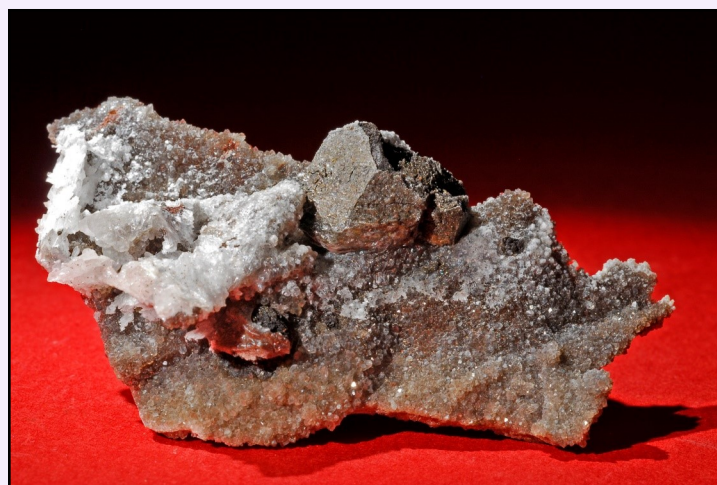
FIGURE 17' DRUSY QUARTZ COATING A FORMER FLUORITE CRYSTAL The white crystalline mass, on the left, is Calcite. (Only small streaks of purple fluorite were found at the mine.)
