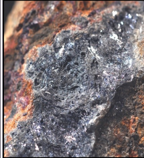
FIGURE 20' GALENA displaying a bright metallic luster, from the north wall of the pit. This galena does not display the typical very good cubic cleavage. This is due, in part, to the presence of silver ions, which tend to disrupt the cleavage planes. This is called argentiferous (silver-bearing) galena. Photo by Stan Celestian
