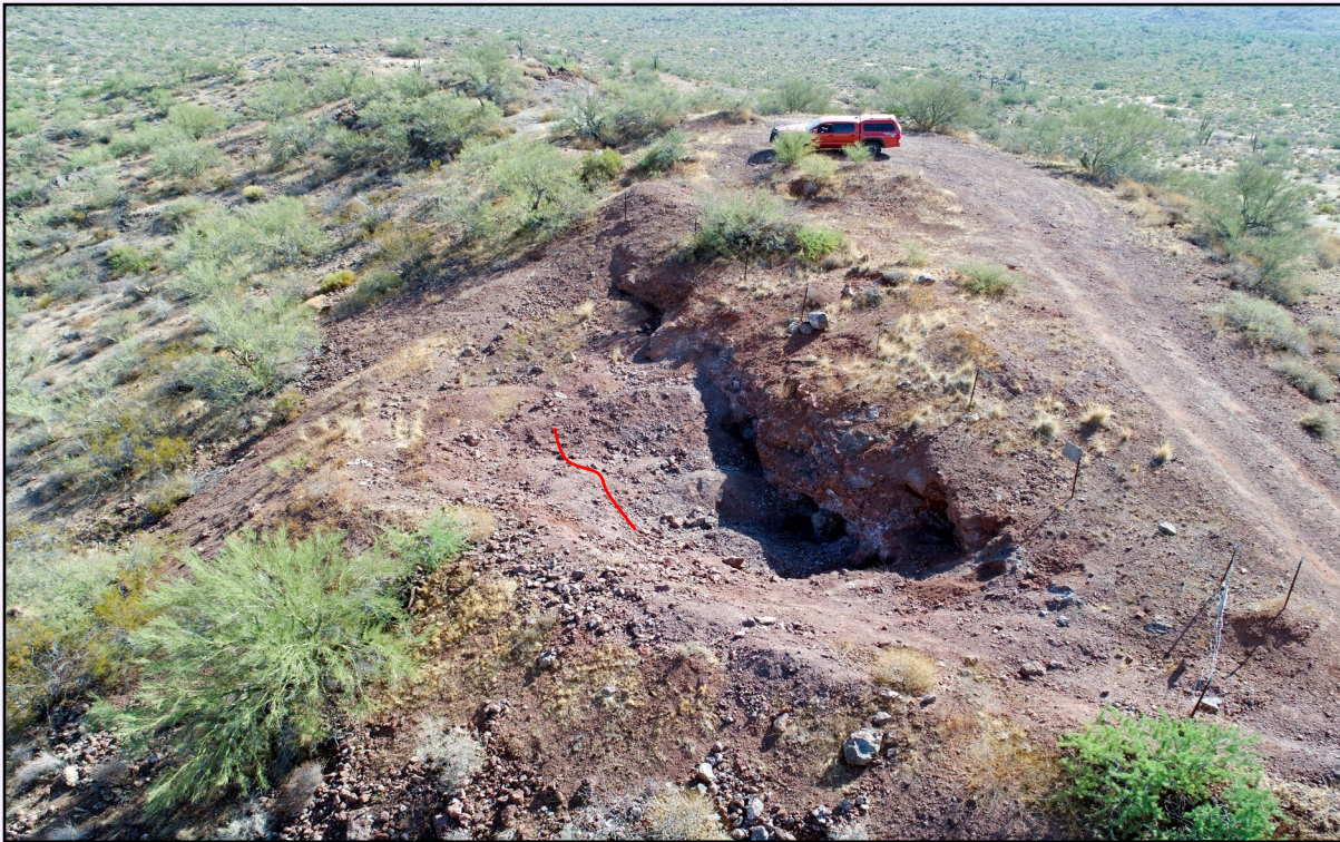
FIGURE 5' This is a closer aerial view of the pit, and also shows the extent of the parking on the hill top. Even from this view, the reddish brown wall rock can be seen. The rock fragments are also visible. The primary ore, galena, was brought into this area by hydrothermal fluids (basically mineral-rich hot water). The fluids moved along a fault line. The fault fragmented the host rock (an igneous rock called diorite). Faulting also opened the rock, so that the fluids could easily move through it. It was along these "water courses" that mineral deposition took place. The red line represents the approximate position of where the galena was found. Well over a hundred pounds of metallic, lustrous galena (PbS) were removed from this area. Another, smaller vein of galena was found near the base of the wall. Veins of barite and quartz can also be found in the wall. Photo by Stan Celestian
