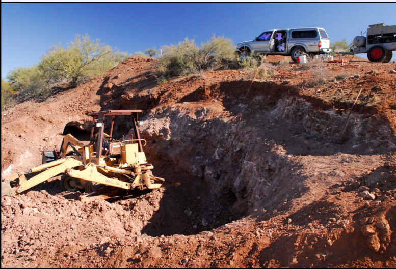
FIGURE 7' Zimmermann provided all of the mining equipment used at the mine. Here he is using a backhoe to muck out an area in the pit. Above the pit is "LeRoi" (LeRoi Airmaster 125 air compressor), a vintage air compressor made in 1942. As you can imagine, getting LeRoi operational was both a science and an art. It came with a hand crank, to get it to turn over. When running, it pumped enough air to operate Zimmermann's 60 pound jackhammer.
