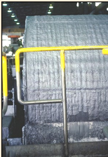
FIGURE 8 DRYER This big rotating dryer (at Bagdad Mine, Yavapai Co., Arizona) sucks the water out of the finely crushed ore. More recently dryers are large tube-like "ovens". From here, ores go to flotation. Photo by Susan Celestian
