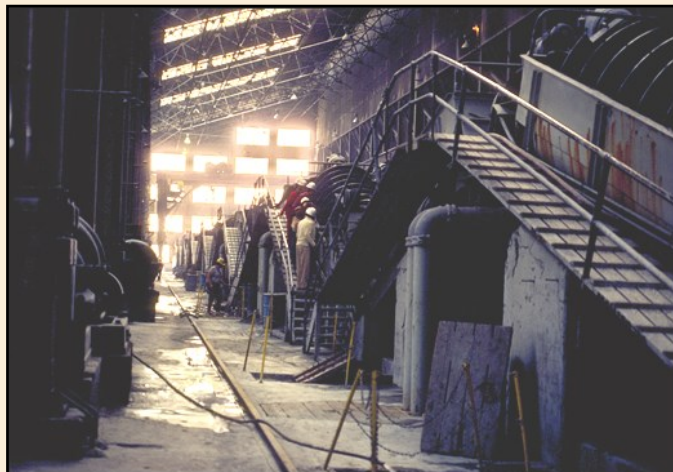
FIGURE 6 MILLS On the left is a ball mill at the Bagdad Mine (Yavapai Co., Arizona) and on the right is a bank of ball mills at the New Cornelia Mine (Ajo, Pima Co., Arizona). After crude crushing, ore rock is sent to the mill and secondary crushers, to be ground to a very fine size. Mills come in three kinds: SAG, ball, and rod.
