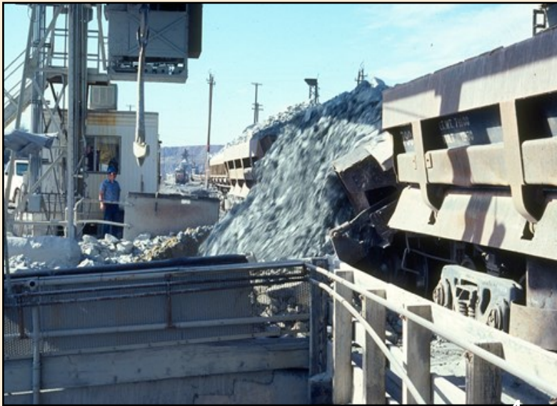
FIGURE 4 PRIMARY CRUSHER AT NEW CORNELIA MINE The crusher is a cone, with a huge concrete pestle, that rotates/gyrates and breaks up rock to 8" or less in diameter.
