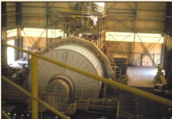
FIGURE 6 MILLS On the left is a ball mill at the Bagdad Mine (Yavapai Co., Arizona) and on the right is a bank of ball mills at the New Cornelia Mine (Ajo, Pima Co., Arizona). After crude crushing, ore rock is sent to the mill and secondary crushers, to be ground to a very fine size. Mills come in three kinds: SAG, ball, and rod.
