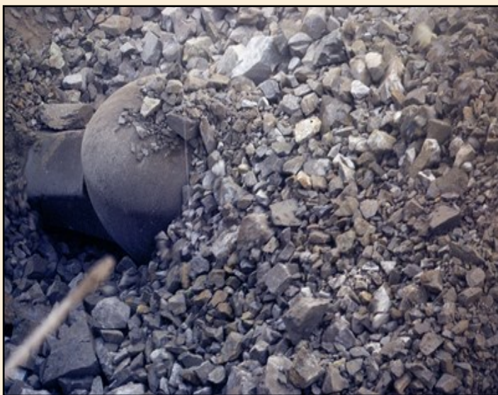
FIGURE 5 ORE IN THE PRIMARY CRUSHER This is a view of the loaded primary crusher in the Bagdad Mine (Bagdad, Yavapai Co., Arizona). From here, the ore is transported via conveyor belt to the ball or rod mills.
