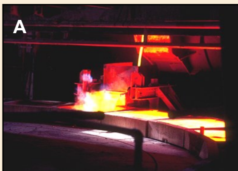
FIGURE 15 POURING COPPER ANODES
