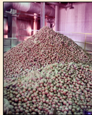
FIGURE 7 RUSTY WORNOUT MILL BALLS at the San Manuel Mine. Photo by Stan Celestian
