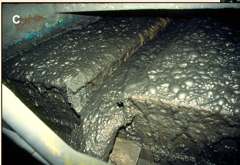
FIGURE 9 FLOTATION OF COPPER ORE The story goes that while hand washing the laundry, women in copper mining camps noticed that copper particles stuck to bubbles in the wash water. And that this observation led to the flotation process. See how coppery the bubbles look!
