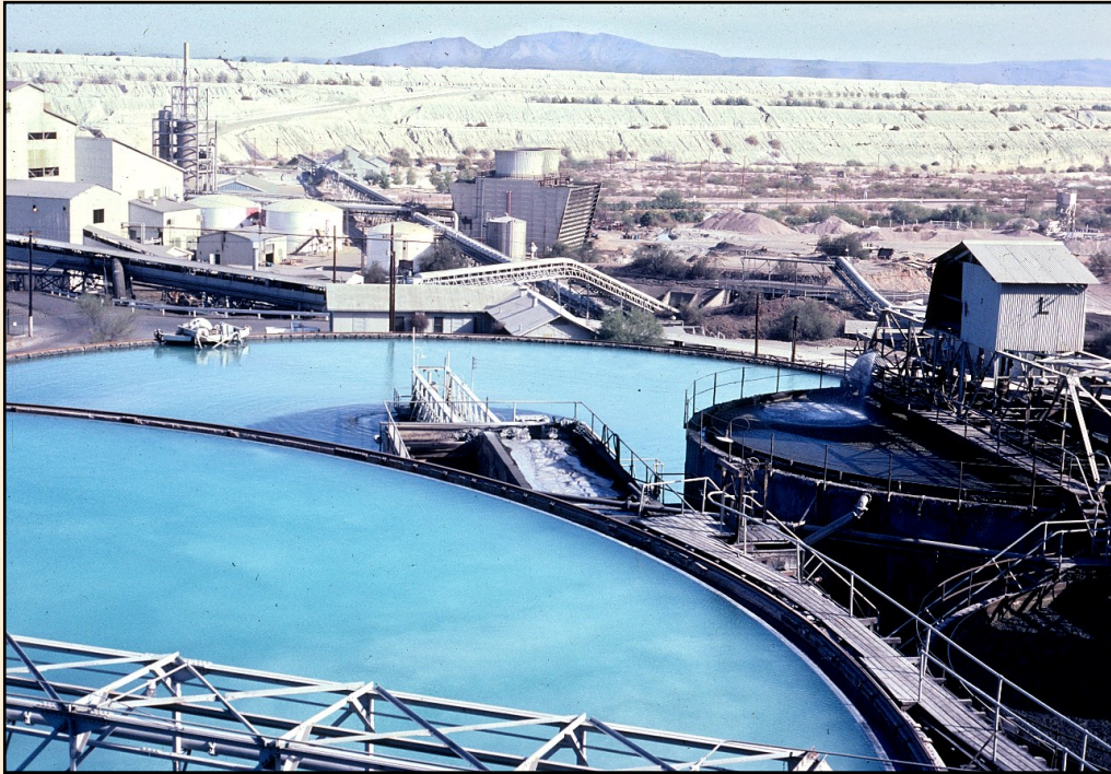
FIGURE 10 TAILINGS (SETTLING) POND AND TAILINGS This photo was taken at the now-closed New Cornelia Mine (Ajo, Pima Co., Arizona). In the foreground is the tailings pond, where tailings settle out of water, and the water is reclaimed. In the background, there is a gray, terraced, and eroded hill. This is where the tailings from the settling pond are dumped. Photo by Stan Celestian
