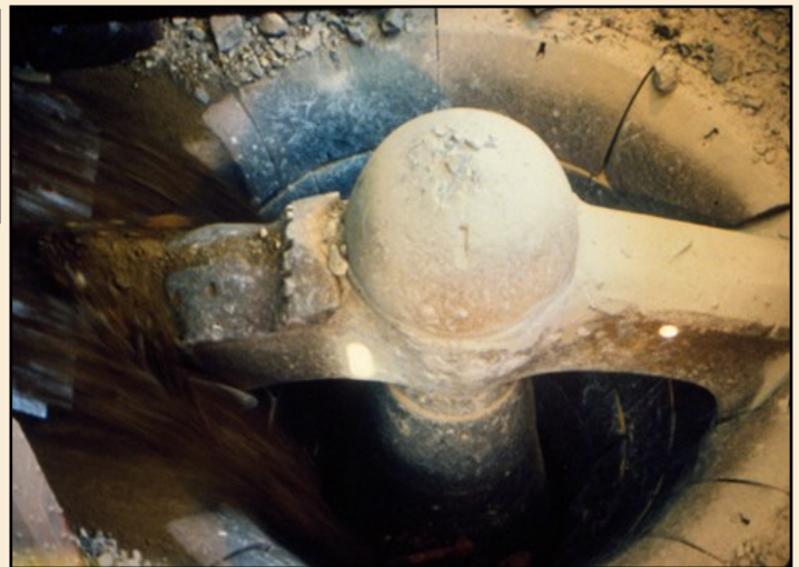
FIGURE 5 ORE IN THE PRIMARY CRUSHER This is a view of the loaded primary crusher in the Bagdad Mine (Bagdad, Yavapai Co., Arizona). From here, the ore is transported via conveyor belt to the ball or rod mills.
