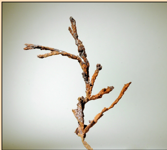
FIGURE 8 NATIVE COPPER Filiform, or thready, habit of copper from the 400' level of the Dugan Mine, Bisbee, Cochise Co., AZ. Photo by Stan Celestian
