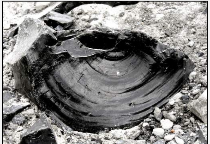
FIGURE DD CONCHOIDAL FRACTURE This glassy, black obsidian is part of the Big Obsidian Flow at Newberry Crater National Park. It exhibits very well developed conchoidal fracture -- a very diagnostic feature.
