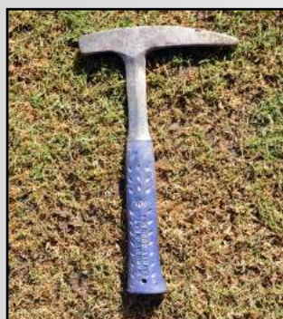
FIGURE 17 GEOPICK This is a tool you can use to pry rocks out of soil, or dig down to them. Never leave home without one. Photo by Stan Celestian
