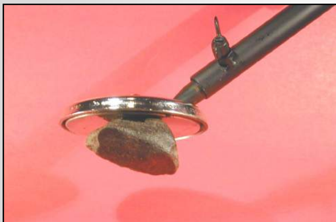
FIGURE 16 STRONG MAGNET As mentioned previously, most meteorites include some iron minerals, and that makes them magnetic (attracted to a magnet). Tool picker-uppers, with strong magnets have a handle and make it easy to sweep the ground for magnetic rocks. Be sure to cover the magnet with a plastic bag, so you don't have to spend hours clearing fine magnetite bits (abundant in Arizona soils) from it. Photo by Stan Celestian
