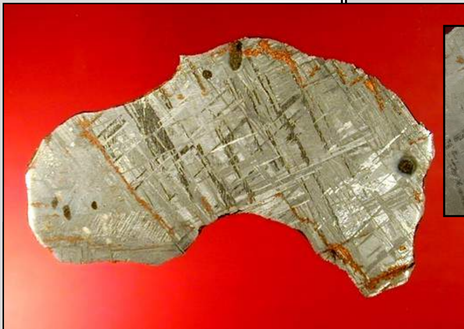
FIGURE 9 WIDMANSTATTEN PATTERN In some types of iron meteorites, long slender nickel crystals are interwoven with ribbons or bands of kamacite and taenite (both alloys of iron and nickel). The pattern is produced by
