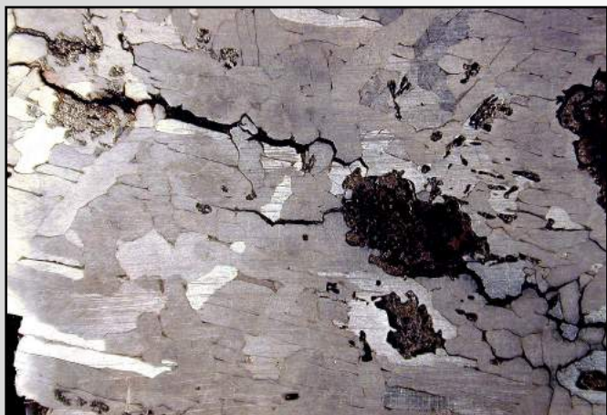
FIGURE 10 WIDMANSTATTEN PATTERN This is the Odessa Meteorite, from Odessa, Texas. Note that the Widmanstätten Pattern is coarser than that of the Gibeon in Figure 9. The black areas are graphite nodules. Photo by Stan Celestian.
