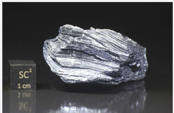
FIGURE B MOLYBDENITE Here are two views of the same specimen of molybdenite. In the lower photo, note the lamellar or layered aspect. It even looks like it feels greasy! Photos by Stan Celestian
