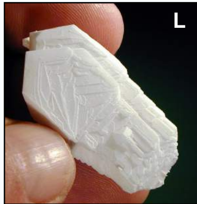
FIGURE 4L MIRABILITE After a couple of hours the crystal from 4J has completely dehydrated, and is now many tiny crystals of thenardite.
