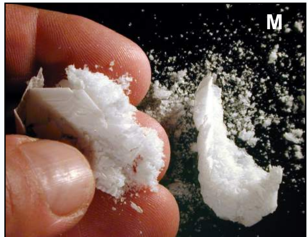
FIGURE 4M MIRABILITE As mentioned in 4L, the once-solid mirabilite crystal has dehydrated and is now composed of many tiny thenardite crystals, making it very fragile. This is the crystal from 4L, after it was gently squeezed. All those tiny thenardite crystals have separated and are scattered about.
