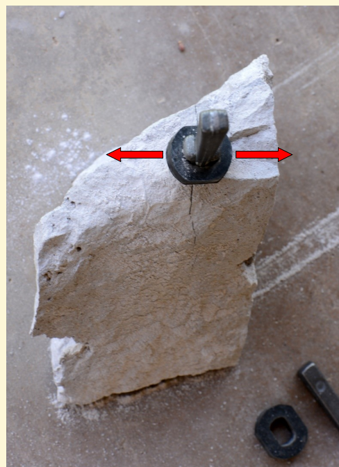
Image 5: The development of a crack created by the hammering of a feather wedge.
