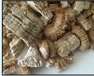
FIGURE 2 EXFOLIATED VERMICULATE Heated vermiculate expands or exfoliates, creating air pockets. Photo by Jungle Rebel and licensed under CC BY 2.0.
