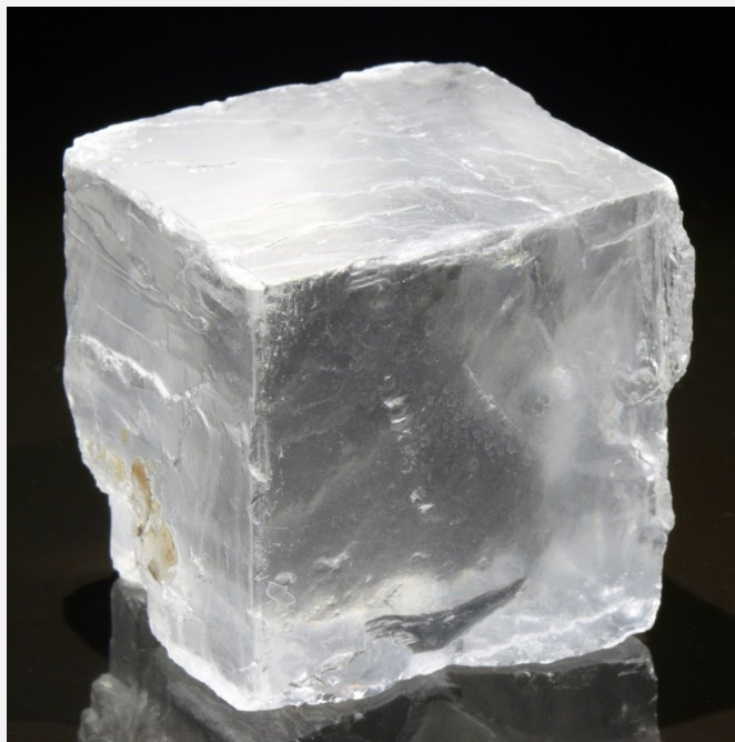
FIGURE 3 CUBIC CLEAVAGE This is a cube of clear halite. It is not a crystal, but a broken chunk, and the perfect cubic cleavage is quite obvious. Photo by Stan Celestian
