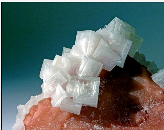
FIGURE 17 HOPPER HALITE Halite tends to grow quite rapidly. As a result, crystal imperfections are common. We've already seen fluids and solids included in crystals. In this instance, the cavernous crystal form is called "hopper". The electrical charge, within the atomic structure, is greatest along the edges (where surface area is greatest); therefore the crystal grows fastest there, leaving the centers of the faces lagging behind. This specimen is from Searles Lake, Trona, San Bernadino Co., CA
