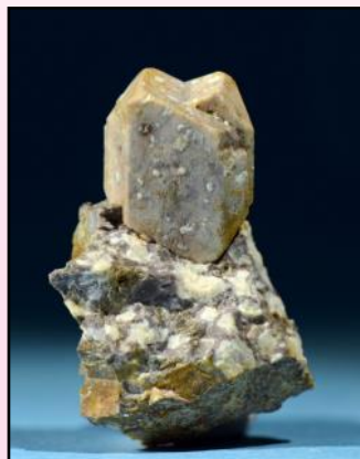
PORPHYRITIC GRANITE - a granite characterized by two distinct grain sizes. In this case the large feldspar crystals within a background of much less coarse crystals of quartz and feldspar. Near Bagdad, Yavapai Co., AZ
