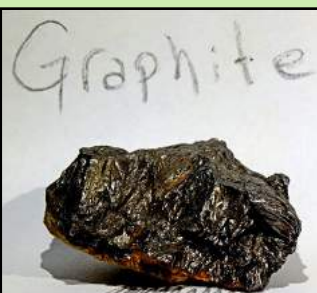
FIGURE 26 GRAPHITE Graphite — the stuff of pencil 'lead — is in lithium batteries Image by Stan Celestian
