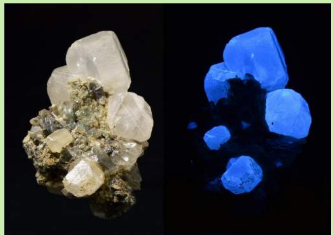
FIGURE 24 TUNGSTEN Scheelite is an ore mineral for tungsten. It fluoresces a rather unique bluish white under SW UV light. UV light is used to both prospect for tungsten, and to sort crushed ore. Images by Stan Celestian and used with permission from the Natural History MUSEUM OF Los Angeles County Gem and Mineral Hall
