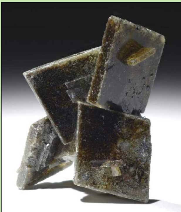
FIGURE 16 BARIUM Barite is the ore mineral for barium, which is a component of insulating materials within smart phones. Image by Stan Celestian From the Magma Mine, Pinal Co., AZ
