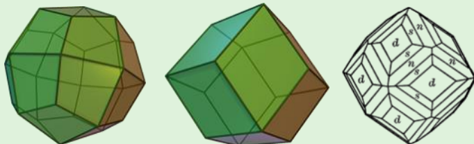
FIGURE 1 COMMON GARNET FORMS Two of the most common forms displayed by garnet are the trapezohedron (on the left) and the dodecahedron (middle). The distinctive faces are a big hint to the identity of garnets in hand specimen. Images by unknown author and licensed under CC BY-SA 3.0
