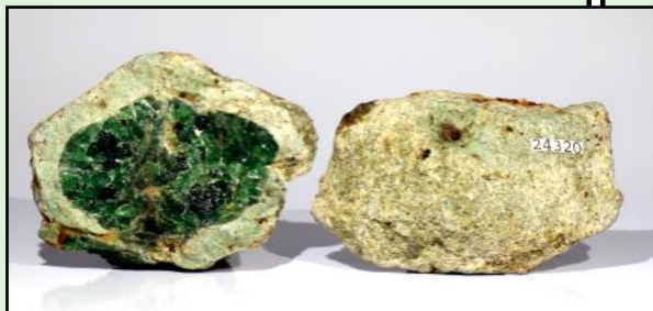
FIGURE 24 GROSSULAR var Tsavorite In Taita Hills, Kenya (in the Tsavo Plains) tsavorite occurs in "potatoes" (porphyroblasts) within a graphite schist. Photos by Stan Celestian and used with permission of the Natural History Museum of Los Angeles County Gem and Mineral Hall.
