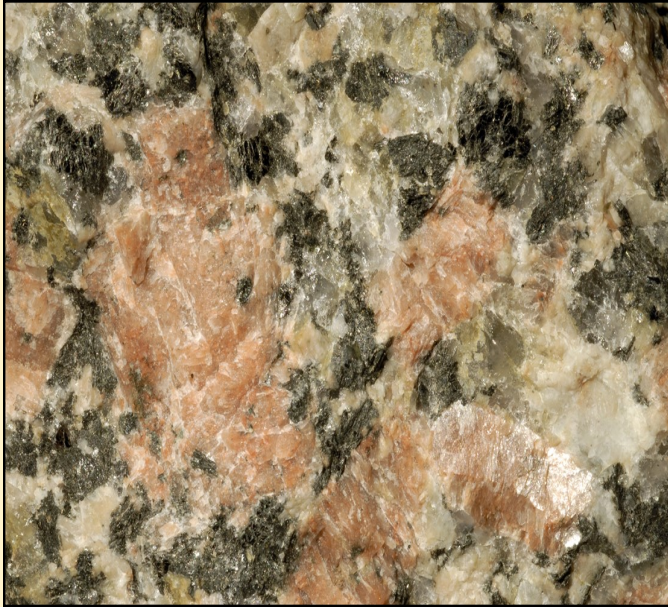
FIGURE 1 Porphyritic Granite In this intrusive rock you can see extra-large rectangular crystals of pink feldspar, surrounded by visible black and white crystals (quartz, feldspar, biotite). Photo by Stan Celestian
