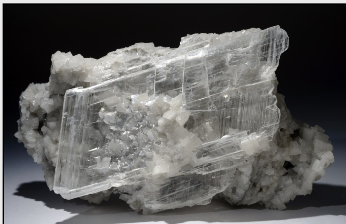
FIGURE B - GYPSUM var SELENITE on DOLOMITE This clear selenite looks sheeted, because gypsum has excellent cleavage along one plane. You could peel this specimen along the cleavage planes, by hand. It is so clear you can see the dolomite crystals behind it. Locality: Lockport Quarry, Lockport, New York Photo by Stan Celestian
