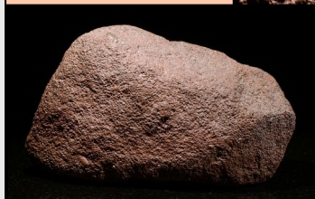
FIGURE F OÖLITIC HEMATITE This form of hematite occurs where hematite precipitates out of a gently agitated
