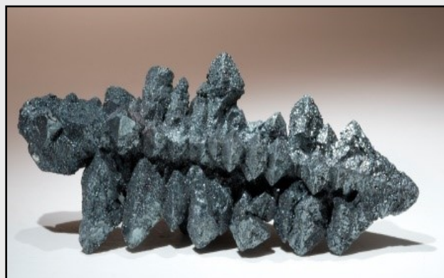
FIGURE H HEMATITE AFTER MAGNETITE This is an aggregate of octahedral magnetite crystals that have been replaced by specular hematite. Photo by Stan Celestian
